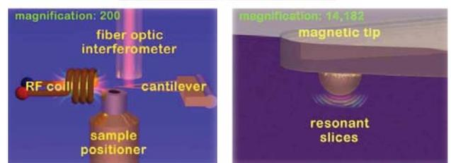
A cantilever with a magnetic tip (center) on
