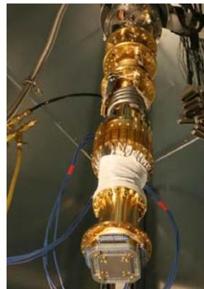
This is the core of a new quantum computer attached to Leiden Cryogenics dilution fridge, ready to begin a cool down to 0.005 degrees above absolute zero... about 500x colder than the coldest place in remote outer space.
